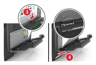
**11** Run the ISP cable through the controller board shield.
