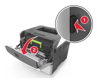
**2** Pull out the toner cartridge using the handle.
