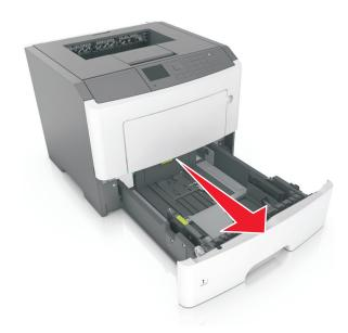
2 Squeeze and then slide the width guide tab to the correct position for the size of the paper you are loading.
