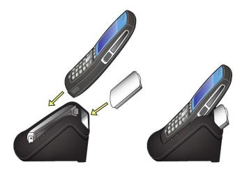
Place the handset in the front slot, facing forward. Battery Packs drop into the rear charging slot.
