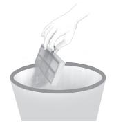
2 Shake off debris by tapping the filter against your trash container.
