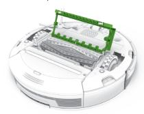
Remove the extractors and remove the yellow extractor caps. Remove any hair or debris that has collected underneath the caps and around the metal axles.
