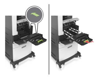
**Note:** Use the arrows on the side of the printer as a guide.
