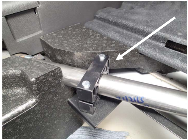
Loosely clamp the hinge / tray assembly to the OEM "X" brace with "V" blocks and 1/4"x 3" Hex bolts. Driver side shown.
