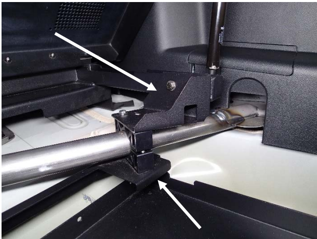
Same mounting for the Passenger side clamp assembly.
