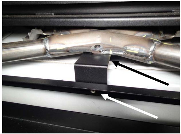
Attach center support bracket to OEM "X" brace with 1/4" x 3/4" hex bolt and fender washer. Attach to tray frame with 1/4" x 3/4" carriage bolt, flat washer and nylon stop nut.
