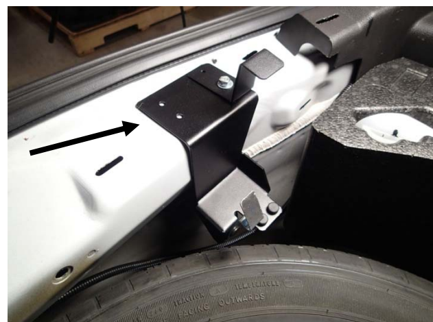
Bolt on the rear latch assembly with 6mm x 16mm hex bolt and washer. Push bracket rearward and tighten. Driver side shown. The C-TTP-INUT-1 bracket shares the same mounting point.
