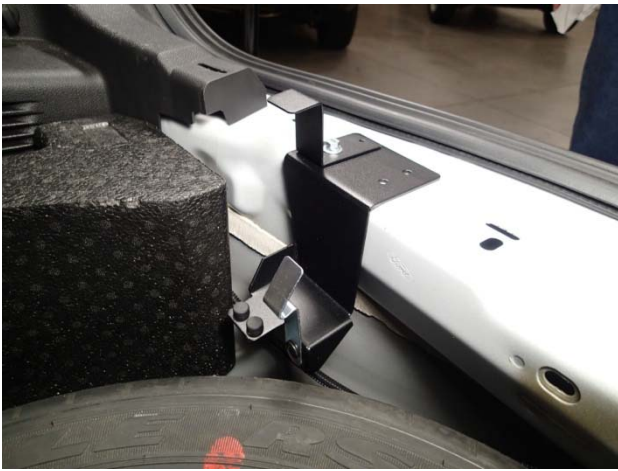
Same mounting for the Passenger side latch assembly.
