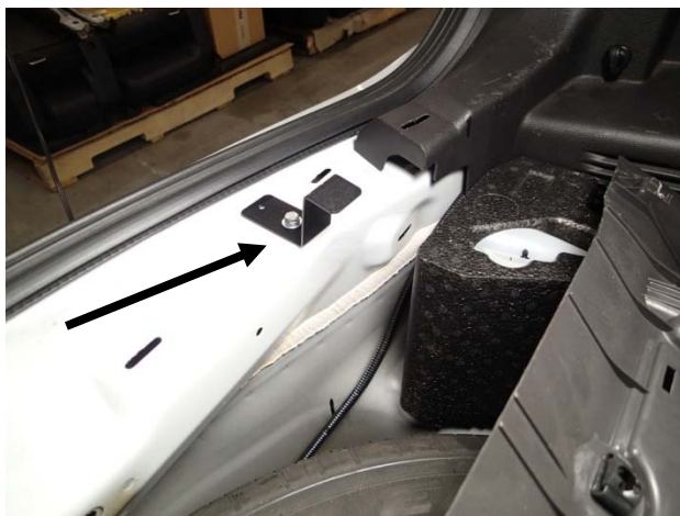
Rear latch brackets use the OEM 6mm threaded holes in the rear door sill.
