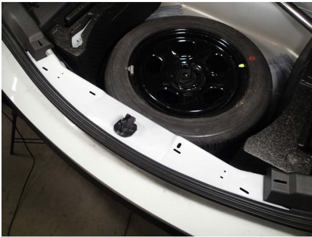
Remove OEM rear sill trim. (Lift up / Unsnap)
