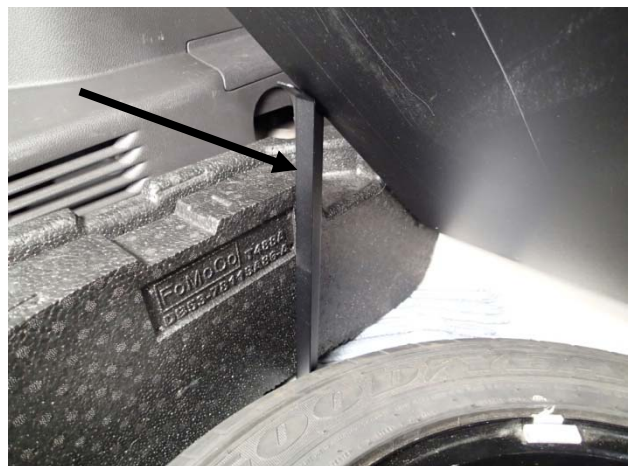
Tray assembly has two props for holding tray up when removing spare tire.
