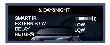
◆ Auto: Automatically, It shifts into the color mode in the bright environment and the B/W mode in the low light condition. It can adjust the delay time, starting brightness and end brightness according to the ambient conditions by pressing the Set button.
