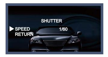
→ INTENSIFY : The brighter image can be displayed by operating digital slow shutter speed in low light environment. (digital slow shutter : x2 ~ x64 // default value : x16)
