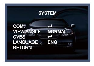
→ CVBS : TV system is manually switchable to 'PAL' or 'NTSC' on CVBS(Composite Video Blanking and Sync).
