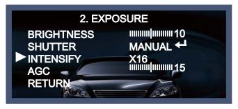
$\rightarrow$  AGC : the brighter image can be displayed by adjusting AGC(Auto Gain Control) level. (AGC : 0 ~ 20 / default : 15 // default value : 15 )
