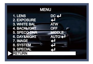
Press 'RETURN' button to save the current settings and exit the setup menu.
