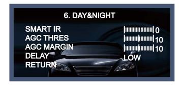
\* SMART IR : It is used to compensate IR saturation  $(0 \sim 20)$
