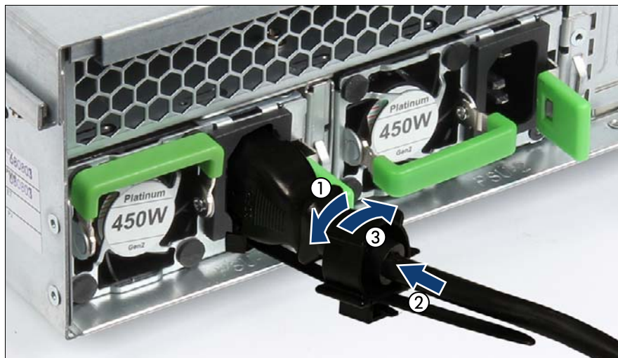
Figure 4: Cable clamp (example AC power supply unit)
