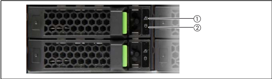
Figure 7: Indicators on the 3.5 inch HDD modules
