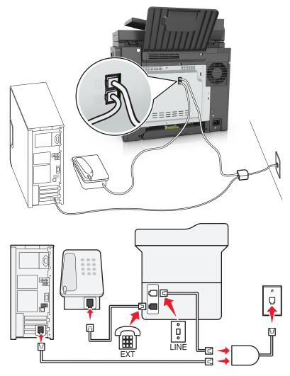
A Digital Subscriber Line splits your regular telephone line into two channels: voice and Internet. Telephone and fax signals travel through the voice channel, and Internet signals pass through the other channel. This way, you can use the same line for analog voice calls (including faxes) and digital Internet access.
