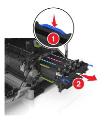
**8** Remove the used developer unit.
