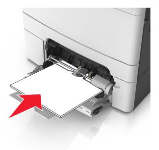
Slide the paper guide until it lightly rests against the edge of the paper stack.
