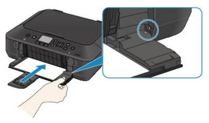
Open the paper output tray, then press the machine's **OK** button.
