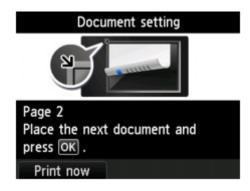
Remove the sheet of original from the platen glass after scanning and load the next sheet on the platen glass, then press the **OK** button.
