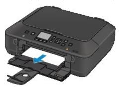
2. Reload the paper, and press the machine's **OK** button.
