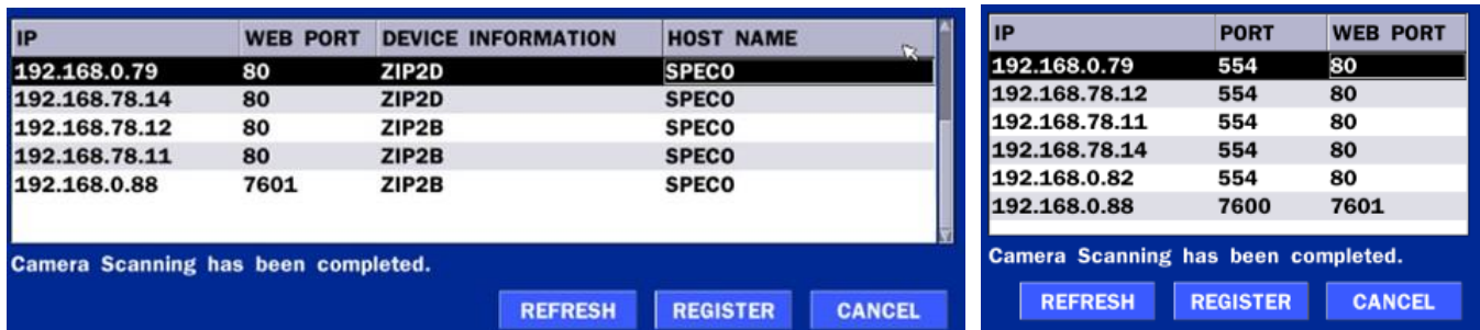
Figure 4.1.3 Left Image using ONVIF Protocol SCAN, Right Image using SPECO Protocol SCAN
