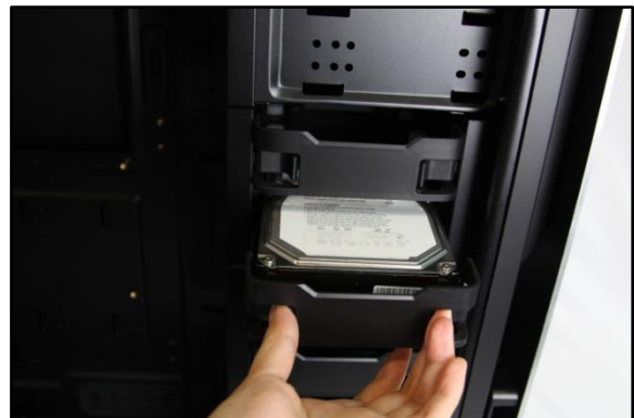
Pinch the ends of the tray and insert your drive until it clicks.
