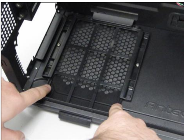
Push down on the ends of the filter to unlock it.
