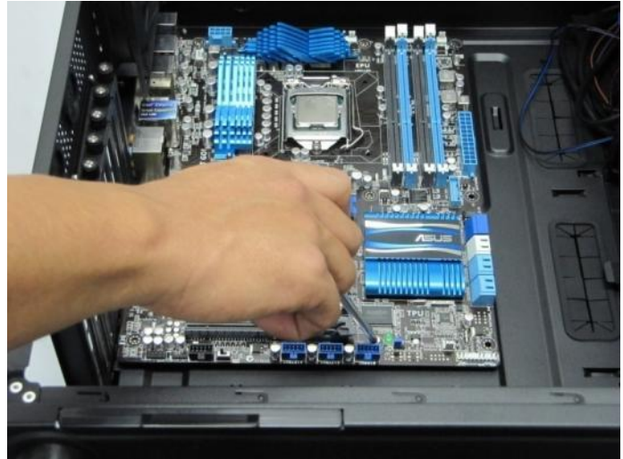
Use the provided motherboard mounting screws to secure your motherboard into the standoffs.
