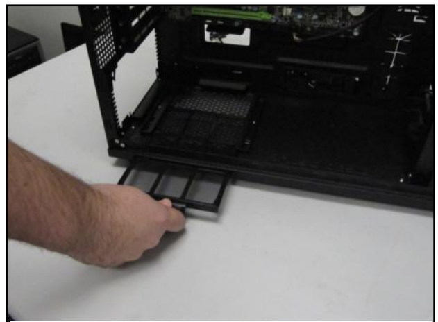
Remove the filter by pulling on the tab outside the chassis.
