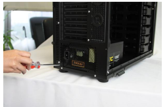
Attach the power supply with the provided screws.
