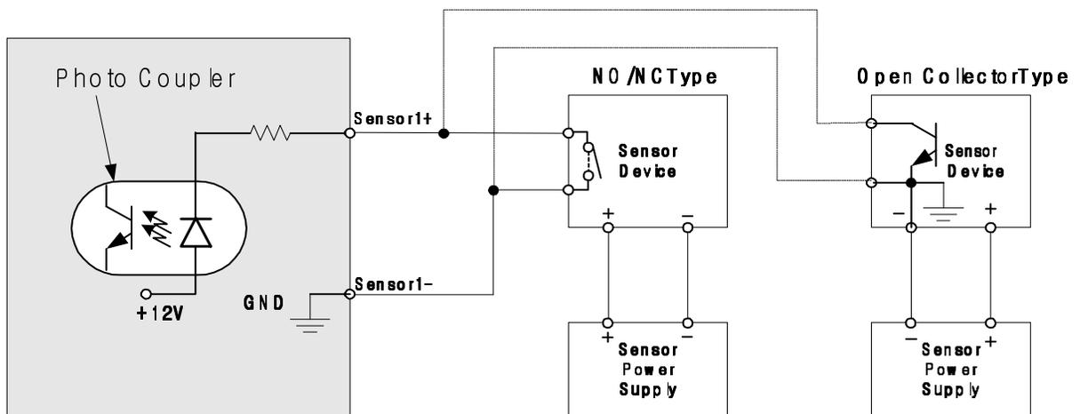
Figure 2-4. SENSOR input and connection of the sensor
