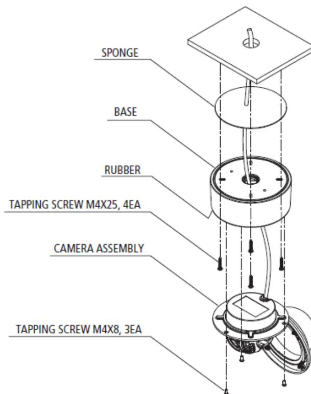
1. Screw the bottom cover to the wall or ceiling by using the mounting screws provided with the camera. Use the mounting template provided with the camera.
