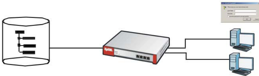
Figure 383 Example: Directory Service Client and Server
