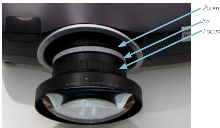
Figure 4-9. Positioning of Zoom, Focus and Iris rings (may vary on some lenses)
