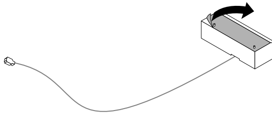
Figure 53. Peeling off the paper that protects the sticker
