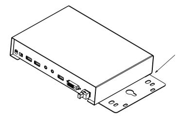
2. Screw the bracket into any convenient location on the rack.
