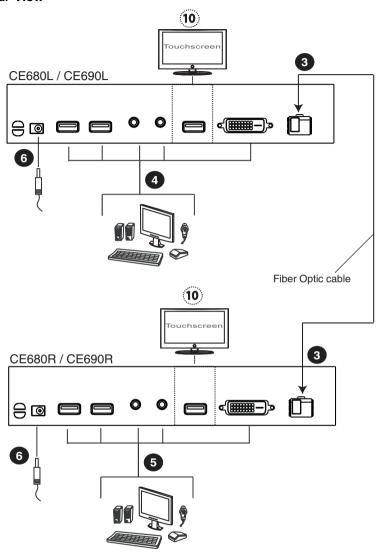
**Note:** The serial port on the CE680L / CE690L connects to the computer; the serial port on the CE680R / CE690R connects to a serial device (optional).
