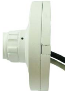
Wire the cables through the wall
