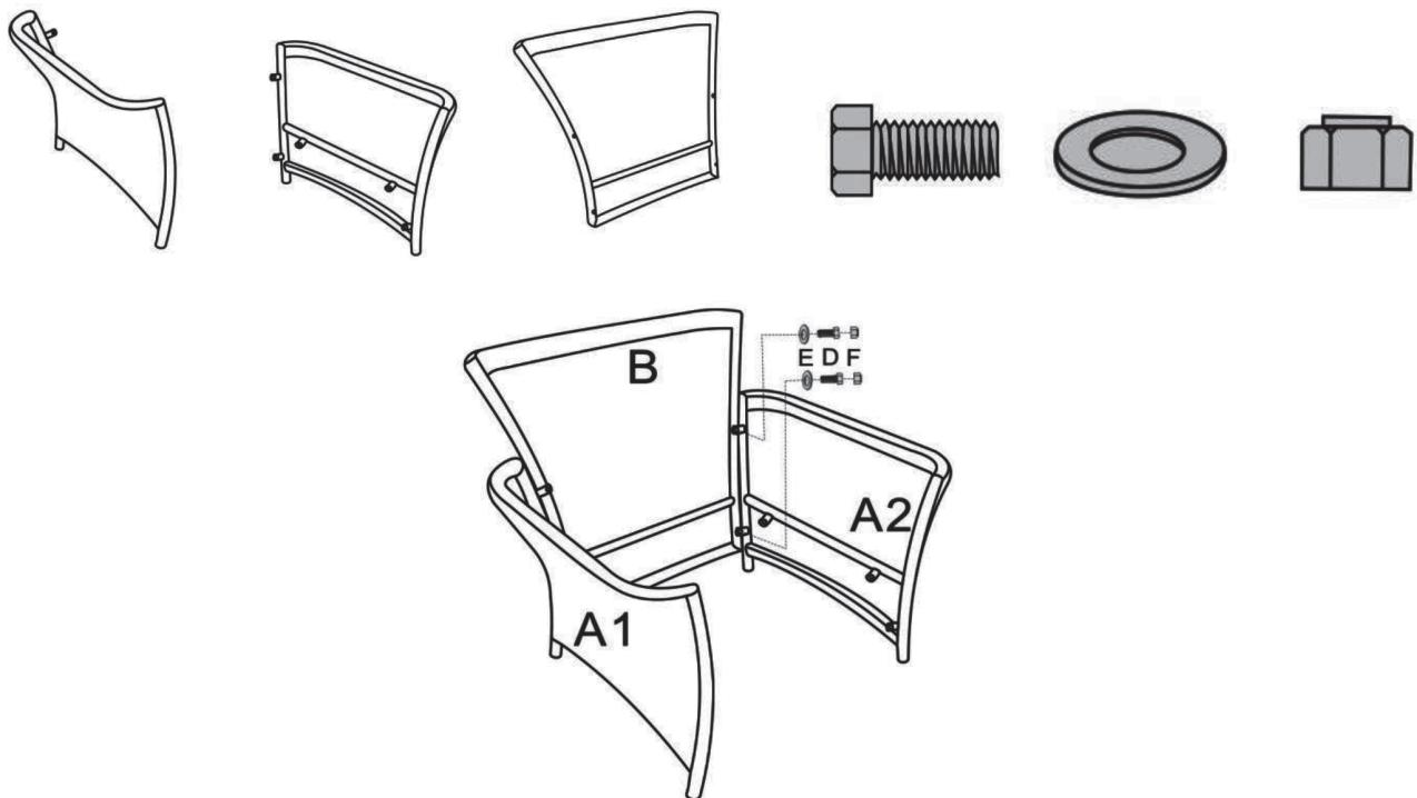
NOTE: DO NOT tighten the bolts completely at this step.
