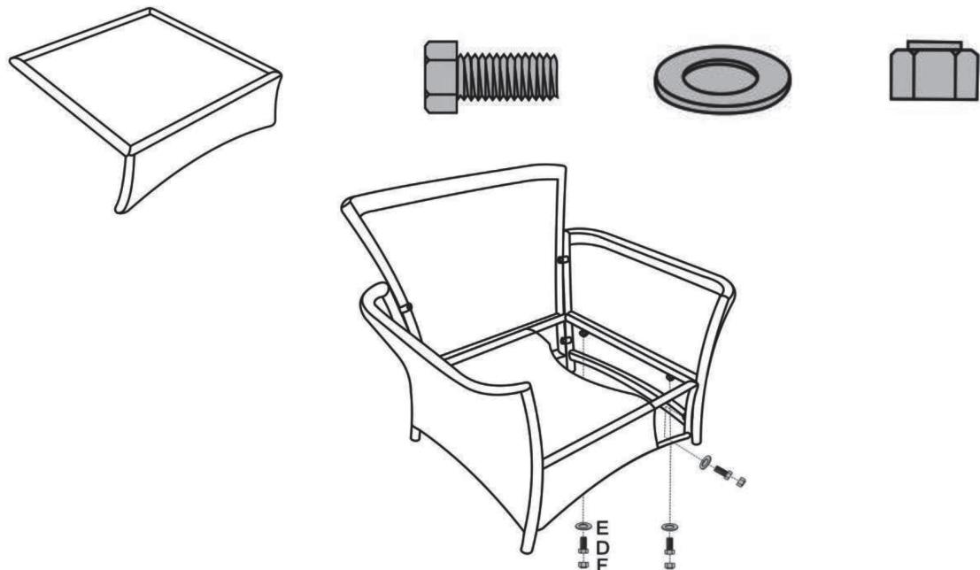
NOTE: Once all bolts are in place tighten completely.
