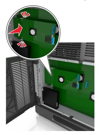
**8** Use the provided thumbscrew for the ISP to attach the plastic bracket to the ISP.
