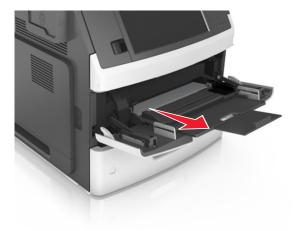
**Note:** Guide the extender gently so that the multipurpose feeder is fully extended and open.
