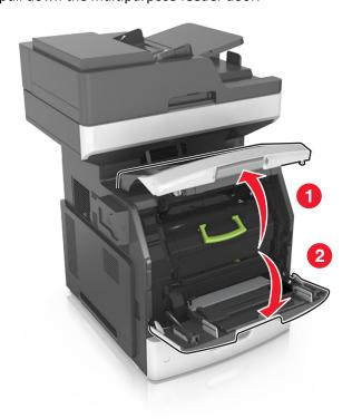
Pull out the toner cartridge from the printer using the handle.
