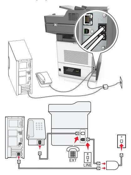
A Digital Subscriber Line splits your regular telephone line into two channels: voice and Internet. Telephone and fax signals travel through the voice channel, and Internet signals pass through the other channel. This way, you can use the same line for analog voice calls (including faxes) and digital Internet access.
