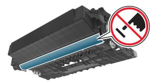
**6** Insert the imaging unit into the printer by aligning the arrows on the side rails of the imaging unit with the arrows on the side rails inside the printer.
