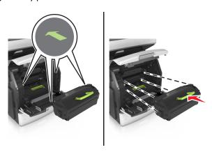
**Warning—Potential Damage:** When replacing a toner cartridge, do not leave the imaging unit exposed to direct light for an extended period of time. Extended exposure to light may cause print quality problems.
