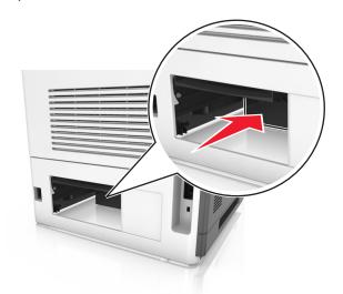
**5** Press down the rear duplex flap, then firmly grasp the jammed paper, and then gently pull the paper out.
