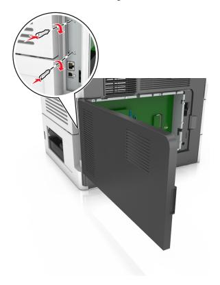
**10** Tighten the thumbscrew that is attached to the ISP.
