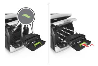
**Note:** Use the arrows on the side of the printer as a guide.
