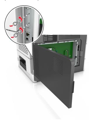
Remove the printer hard disk.
