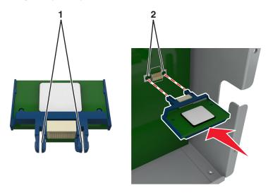
**4** Push the card firmly into place as shown in the illustration.
