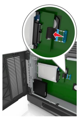
Remove the screws holding the printer hard disk in place.
