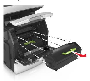
**3** Unpack the new toner cartridge, then remove the packing material, and then shake the cartridge to redistribute the toner.
