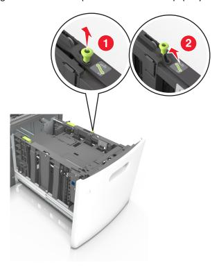
**b** If the A5 length guide is still attached to the length guide, then remove it from its place. If the A5 length guide is not attached, then proceed to step d.
