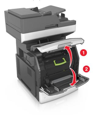
**2** Pull the cartridge out of the printer using the handle.
