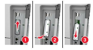
**5** Align the posts of the plastic bracket to the holes on the controller board cage, and then press the plastic bracket on the controller board cage until it *clicks* into place.
