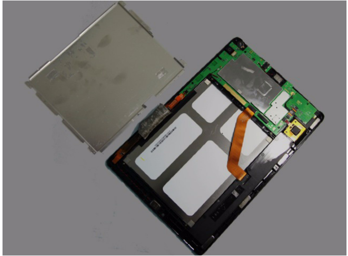
Figure 3-3. The removed battery holder
