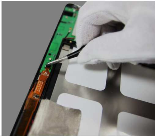
Figure 6-1. Peeling off the mylar on the CAP sensor FPC connector
