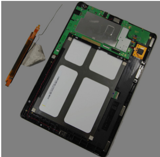
Figure 6-10. Removing the antenna and CAP sensor FPC assembly
