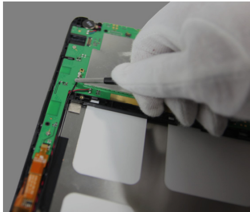
Figure 6-8. Taking out the RF cable from the cable duct
