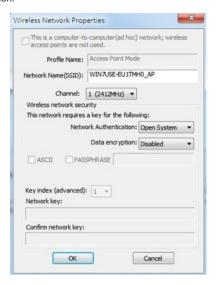
Network Name (SSID) - The network name of the AP, searchable by other wireless nodes. The length of SSID should be shorter than 32 characters.
