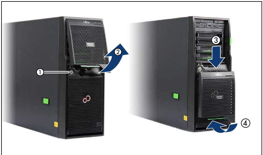
Figure 5: Removing the drive cover and placing it on the HDD cover
