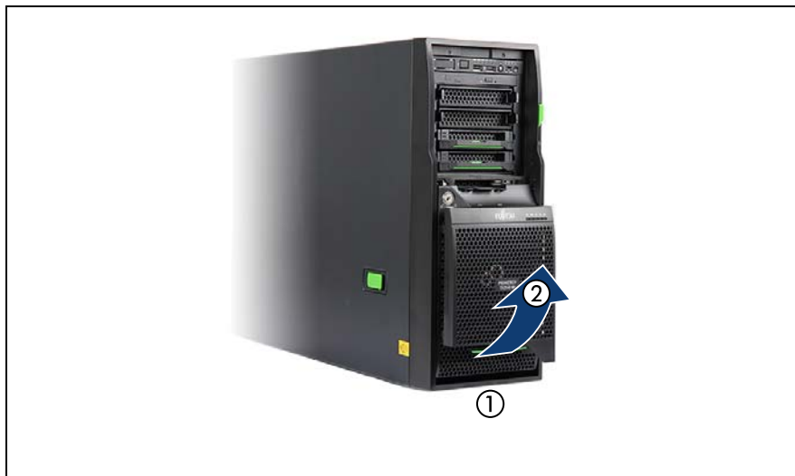
Figure 6: Removing the drive cover from the hard disk drive cover
