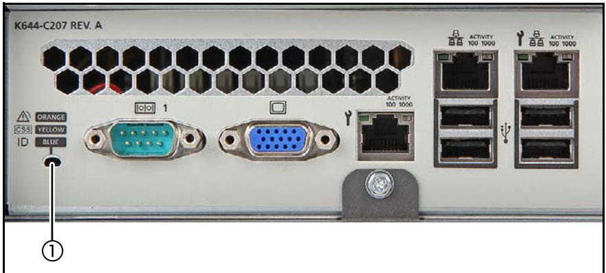
Figure 12: Indicator on the connection panel: CSS, Global Error and ID indicator
