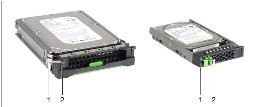
Figure 10: Indicators on the 3.5 inch and 2.5 inch HDD modules
