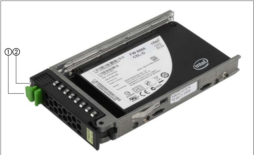
Figure 11: Indicators on the SSD modules
