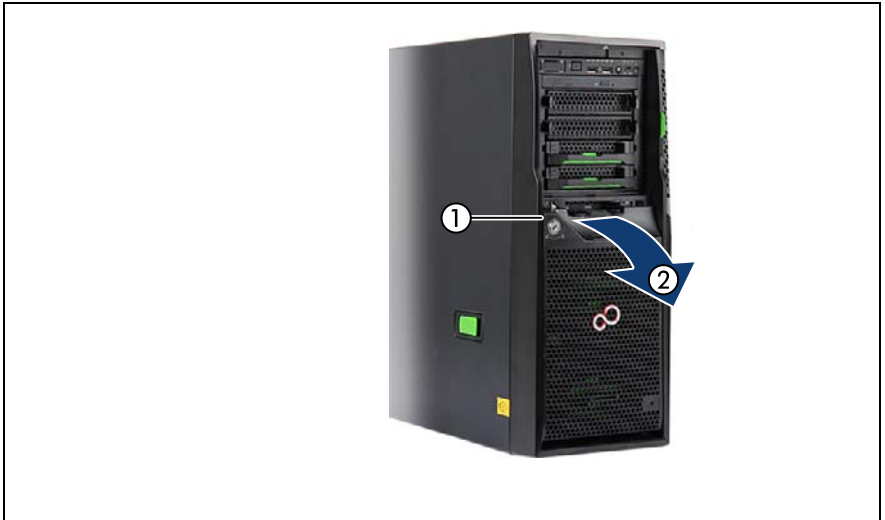
Figure 7: Removing the hard disk cover
