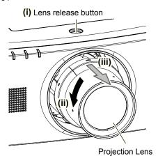
1) With the lens release button held down, turn the Projection Lens counterclockwise to the end and remove the Projection Lens.
