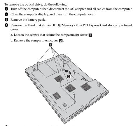
**5** Remove the screw shown in the illustration **3**.
