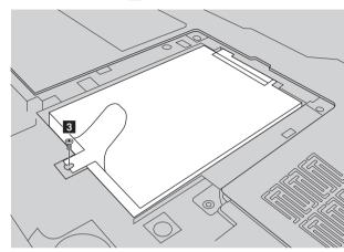
**5** Remove the frame fixing screw **3**.
