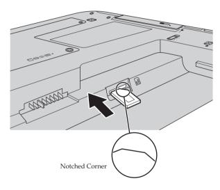
**5** Put the battery back in place. Turn the computer over and reconnect the cables.
