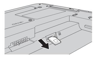
**5** Put the battery back in place. Turn the computer over and reconnect the cables.
