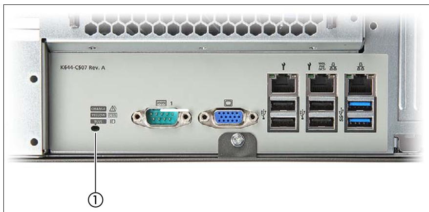
Figure 11: Indicators on the connector panel: CSS, Global Error and ID indicators
