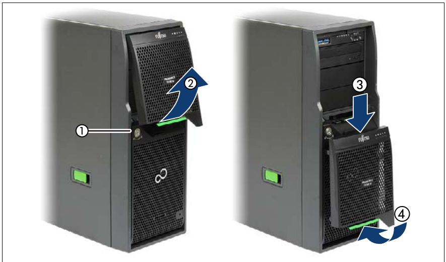
Figure 5: Removing the drive cover and snapping it into the HDD cover
