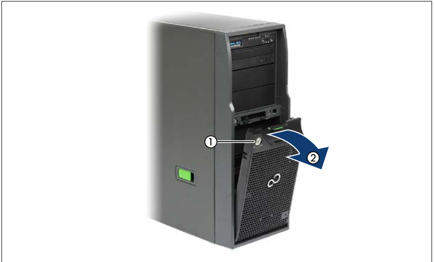
Figure 7: Removing the HDD cover
