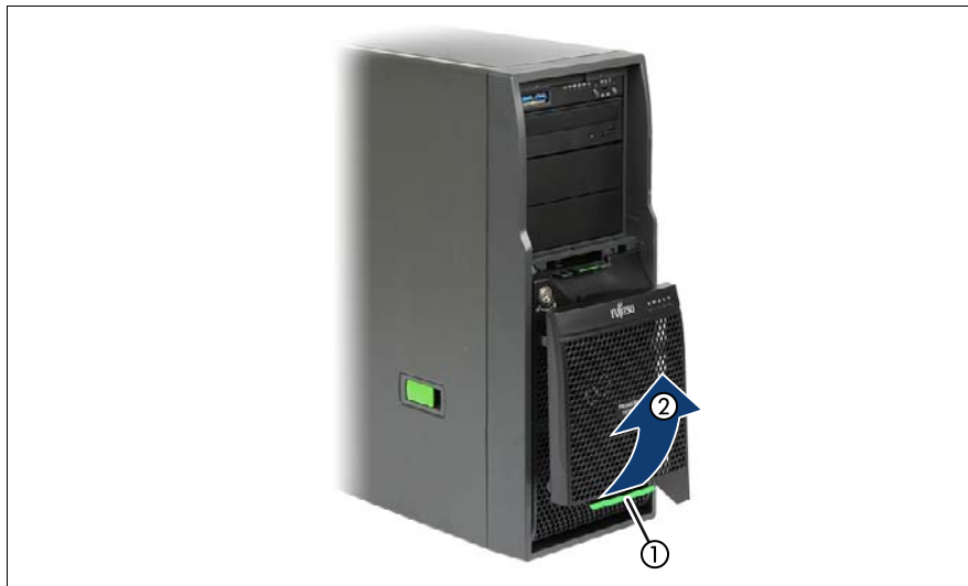
Figure 6: Removing the drive cover from the HDD cover
