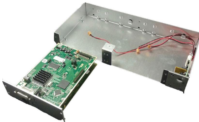
Figure 3-8. Example of a 4-Port chassis that shows three power connections.
