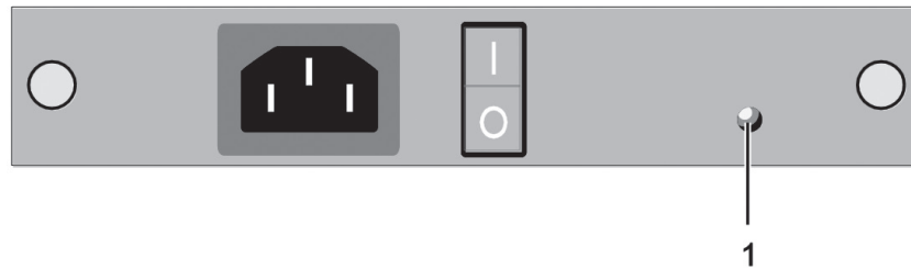
FIGURE 2-13. STATUS LED ON THE POWER SUPPLY UNIT
