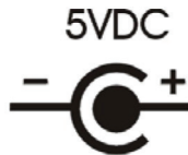
Figure 1-8. Power supply label.
