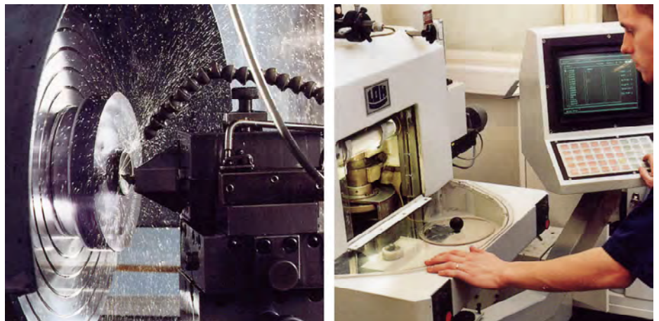
Figure 14.4 LEFT: Diamond turning machine; RIGHT: Lens polishing
