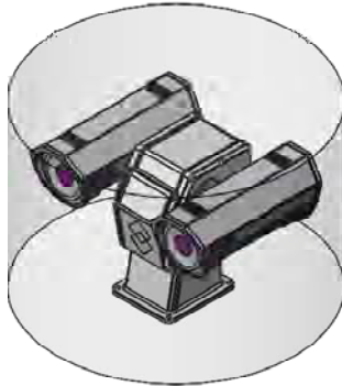
Figure 7.2 FLIR A3xx pt series camera exclusion zone. Height 480 mm (18.9"), diameter 740 mm (29.1").
