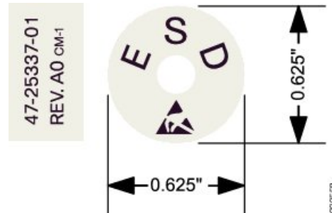
Figure 2: ESD Label Information on Cisco ASR 9910 Router Chassis
