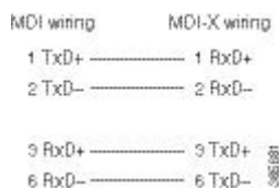
Figure 65: Straight-Through Cable Pinout to a Hub, Repeater or Switch
