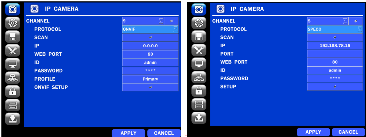
Figure 4.1.2 IP CAMERA Setup Screen
