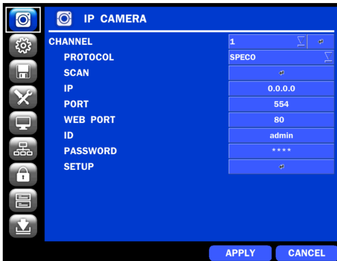
Figure 4.1.1. IP Camera mode setup screen
