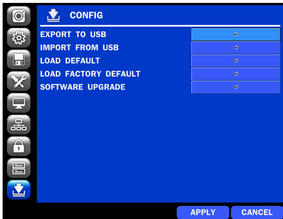
Figure 4.9.1. CONFIGURATION Setup Screen
