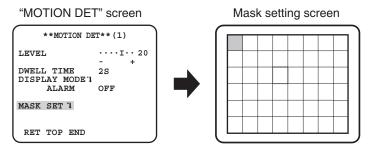
In the masked area, no alarm will be issued even if a moving object is detected. The masked area is set in the same way as the masked area setting in "Light quantity control method selection". (1287 page 13)
