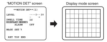
Move the cursor to "LEVEL" and press the [RIGHT] or [LEFT] button to adjust the level. Repeat step 5 and 6 to adjust to optimal level.
