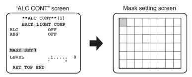
Press the [UP], [DOWN], [RIGHT], and [LEFT] buttons to move the flashing cursor to the area to be masked and press the [SET] button.
