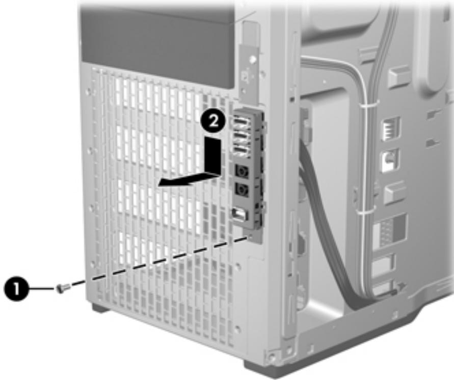
9. Disconnect the speaker cable (see [Removing the speaker on page 87](#)), and remove the tie wraps that secure the front panel I/O cables to the chassis.
