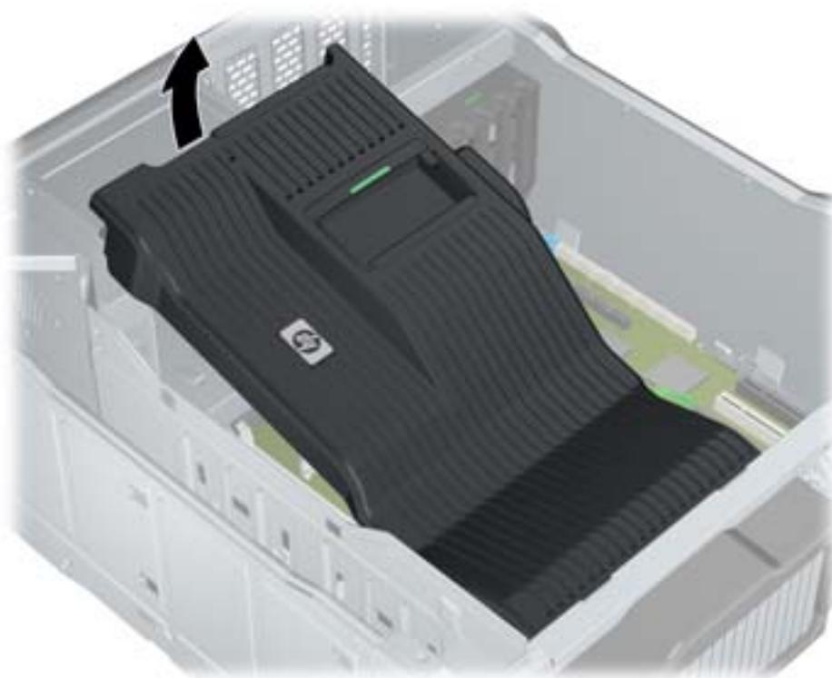
4. Remove the LCS air duct from the airflow guide.
