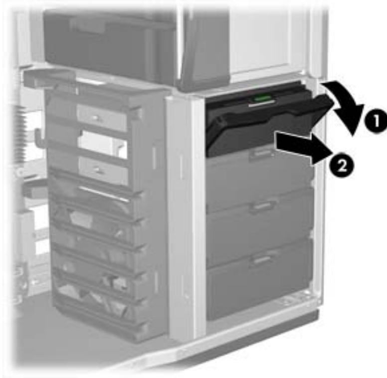
5. Set the hard drive in the carrier at an angle. Carefully separate the lower hard drive carrier rails (1), and then lower the drive between them, as shown in the following figure.
