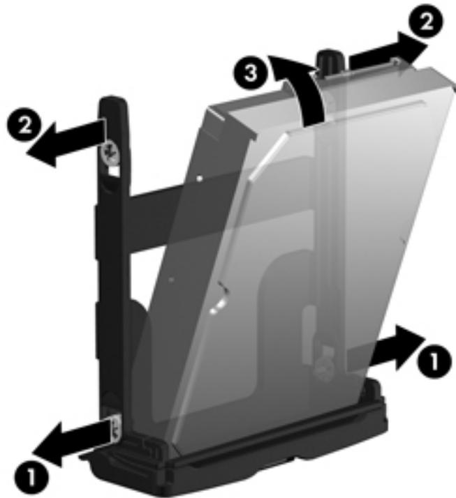
6. Carefully separate the upper hard drive carrier rails (2), and then rotate the drive upright (3), as shown above.
