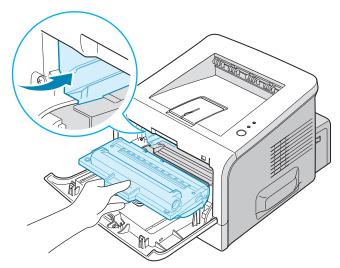
**5** Grasp the handle and insert the cartridge into the printer until it snaps into place.
