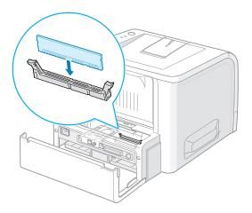
6 Hold the PS DIMM so that the notch and the connection point are aligned with the slot as shown, and insert it all the way into the lower slot.
