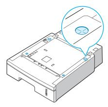
4 Align the printer with the support unit and lower it into place on the tabs.
