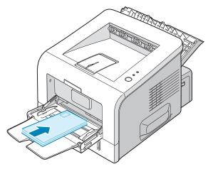
**5** Adjust the guide to the edge of the envelope stack.
