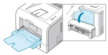
**2** Load transparencies with the print side up, and the top with the adhesive strip entering the printer first.
