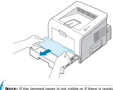
**NOTE:** If the jammed paper is not visible or if there is resistance when you pull the paper, remove the tray from the printer and carefully pull the jammed paper free from the printer.
