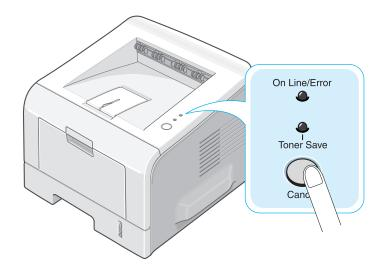
The printer will finish printing the page that is moving through the printer and delete the rest of the print job. Pressing the button cancels only the current job in the printer. If more than one print job is in the printer memory, the button must be pressed once for each job.
