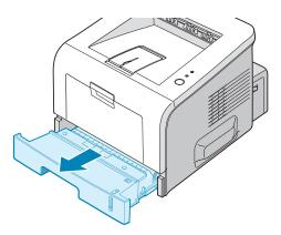
**2** Prepare a stack of paper for loading by flexing or fanning the paper back and forth. Straighten the edges on a level surface.
