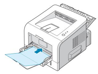
3 Adjust the guide to fit the width of the material stack.
