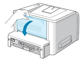
**CAUTION:** The fusing area at the rear portion of the inside of your printer is hot when powered. Be careful not to be burned when accessing this area.
