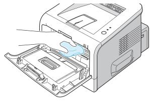
**NOTE:** To prevent damage to the toner cartridge, do not expose it to light for more than a few minutes. Cover it with a piece of paper, if necessary and keep it in a flat and clean place. Also, do not touch the black transfer roller inside the printer.
