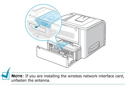
6 Make sure that the connector on the card is properly placed on the connector of the board. Push the card firmly.
