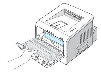
**CAUTION:** To prevent damage to the toner cartridge, do not expose it to light for more than a few minutes. Place a piece of paper over the top of the toner cartridge to shield it while it is out of the printer and keep it in a flat and clean place.
