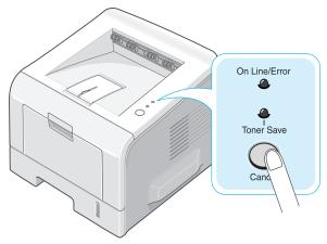
3 Your printer automatically picks up a sheet of paper from the tray and prints out a cleaning sheet with dust or toner particles on it.
