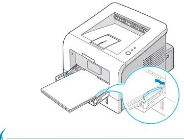
**NOTE:** Your printer cannot automatically detect the size of paper loaded in the Multi-Purpose Tray. Loading the Multi-Purpose Tray with the correct paper size allows you to select paper by size rather than paper source when you print from your software application. You do not have to check which paper is loaded in the Multipurpose Tray before printing.
