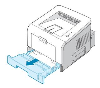
2 Remove any misfed paper by pulling it out by the visible edge. Make sure that all of the paper is properly aligned in the tray.
