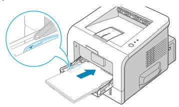
If you want to print on previously printed paper from the Multi-Purpose Tray, the printed side should be facing down with an uncurled edge to the printer. If you experience problems with paper feed, turn the paper around.
