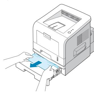
**3** If you cannot find the jammed paper in Tray2, pull Tray1 half way out of the printer, and remove the paper.
