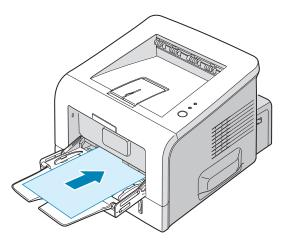
2 Slide the paper width guide and adjust it against the material without bending.
