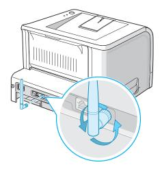
**11** Plug one end of the Ethernet cable into the Ethernet network port on the Printer and the other end of the cable into a network LAN connection.
