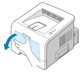
2 Unfold the extender to extend the tray to its full-length to hold longer paper.
