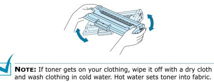
4 Reinsert the toner cartridge into the printer. Ensure that the toner cartridge snaps into place.
