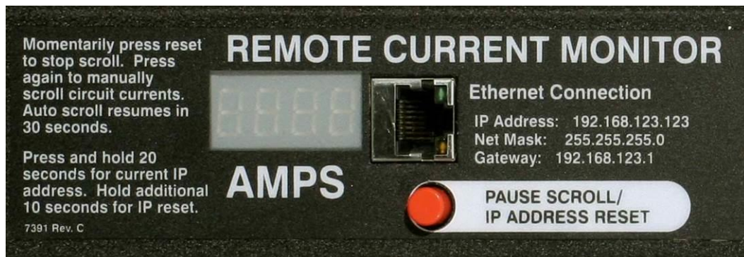
Current Monitoring Meter
