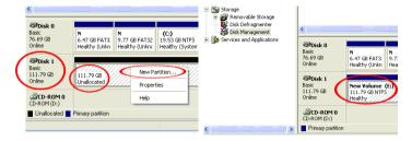
If you are installing a hard drive that already has data on it, then after plugging it in, the drive should automatically show up with a drive letter assigned within My Computer.
