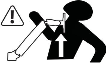
**EN** WARNING! Stored Energy Hazard: The arm mechanism is under tension and will move up rapidly, on its own, as soon as attached equipment is removed. For this reason, DO NOT remove equipment unless the arm has been moved to the highest position! Failure to follow this instruction may result in serious personal injury and/or equipment damage!
