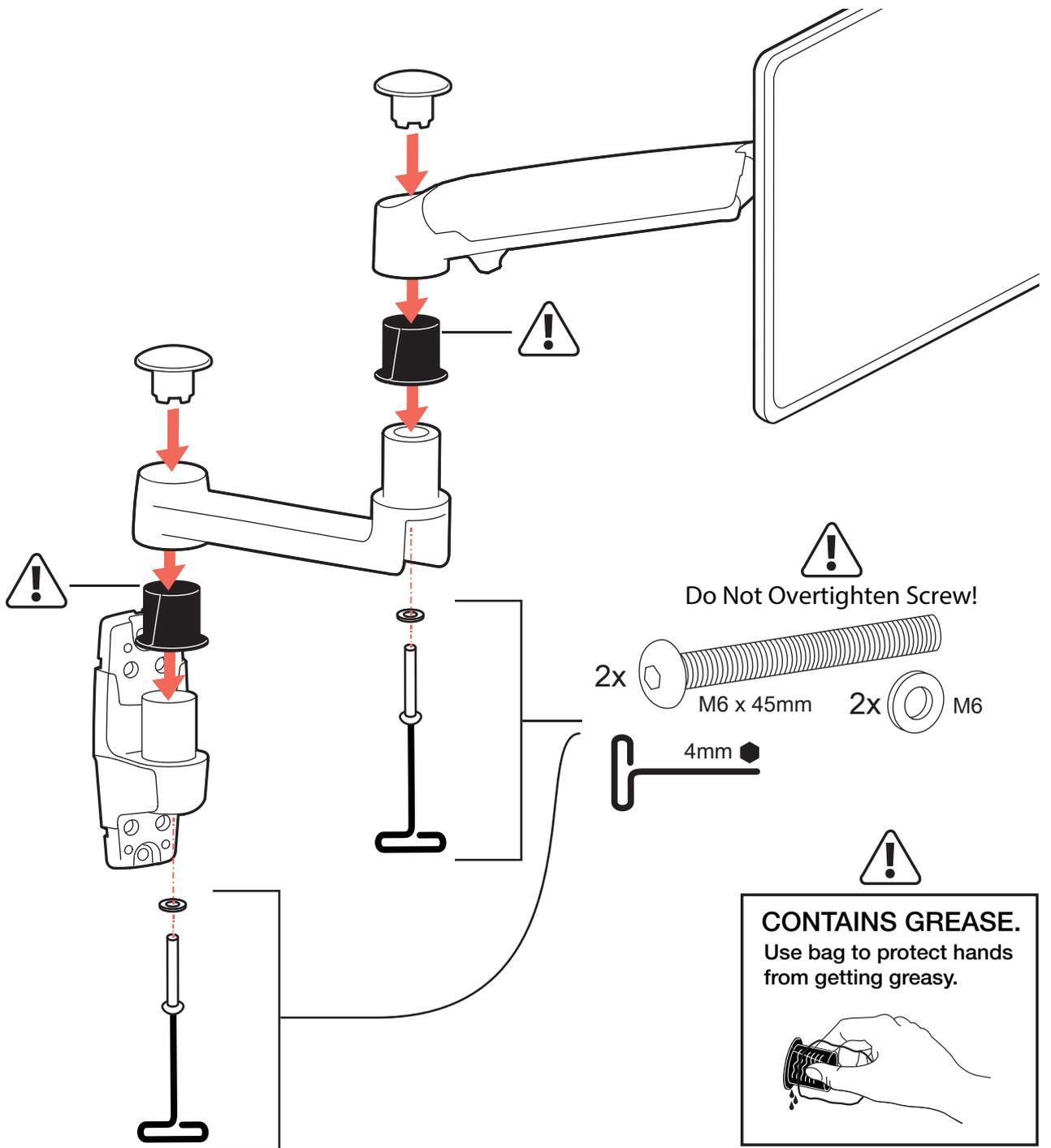
NOTE: when sliding sleeve on to bracket, align slot over rotation stop.
