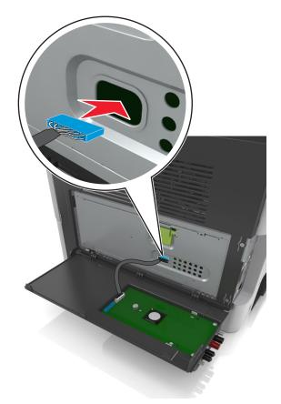
**11** Open the controller board shield using the green handle.
