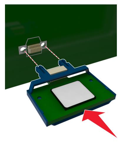
**Warning—Potential Damage:** Improper installation of the card may cause damage to the card and the controller board.
