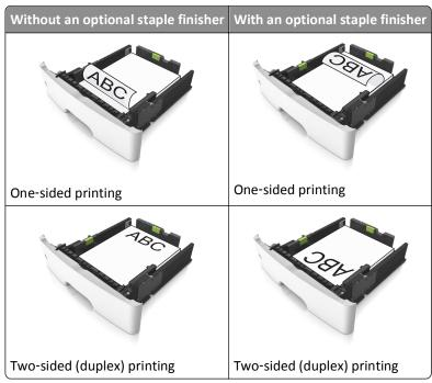
• Make sure the paper is below the maximum paper fill indicator located on the side of the width guide. Overfilling may cause paper jams.
