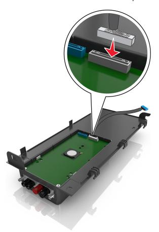
Slightly close the ISP exterior cover up to 65 degrees, and then slide the cover to attach.
