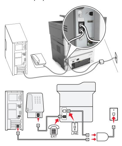
A Digital Subscriber Line splits your regular telephone line into two channels: voice and Internet. Telephone and fax signals travel through the voice channel, and Internet signals pass through the other channel. This way, you can use the same line for analog voice calls (including faxes) and digital Internet access.
