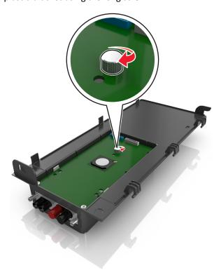
Tighten the two screws on the end of the ISP solution.
