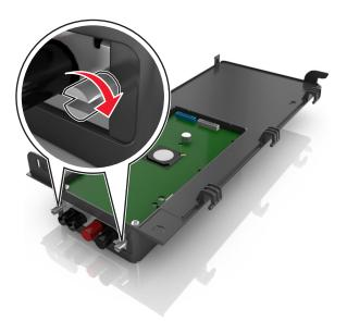
Attach the white plug of the ISP solution interface cable into the white receptacle on the ISP.
