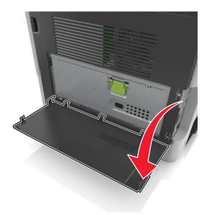
2 Lightly press the stop on the left side of the controller board access door, and then slide the access door to remove.
