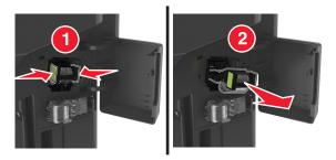
$\textbf{3} \quad \text{Hold both sides of the empty staple case with your fingers, pull, and then lift the empty staple case from the cartridge.}$
