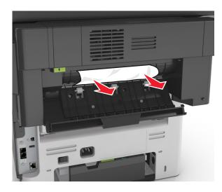
**3** Open the finisher trap door, remove any paper fragments inside the trap door.
