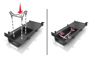
Slide and push the ISP solution into the plastic bracket.
