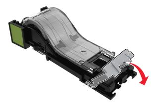
Insert stapler cartridge back into the finisher until it *clicks* into place.
