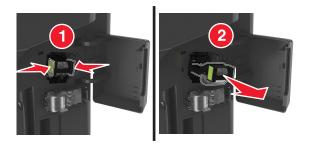
Lift the staple guard, and then remove any jammed or loose staples.
