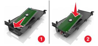
Secure the ISP solution to the plastic bracket using the long screw.
