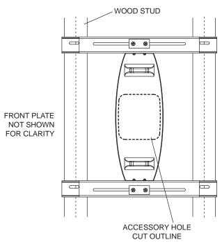
Attach surge protector (**B**) to outlet box (**C**) and in-wall box (**A**) with four #6 x 3/8" screws (**D**). **NOTE:** Service of an electrical gang box and wiring shall be performed by a qualified service personnel in accordance with the NEC.
