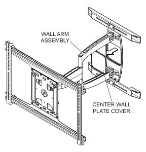
Use wall arm assembly as a template to draw outline of accessory hole as shown below. Remove drywall inside cut outline.
