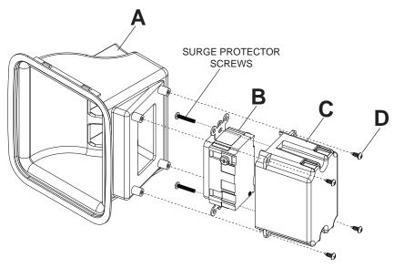
Insert in-wall box (A) through accessory hole in left or right position.
