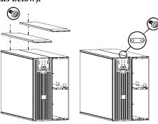
2. Install the tie bracket securing the UPS and external battery pack (screws included).
