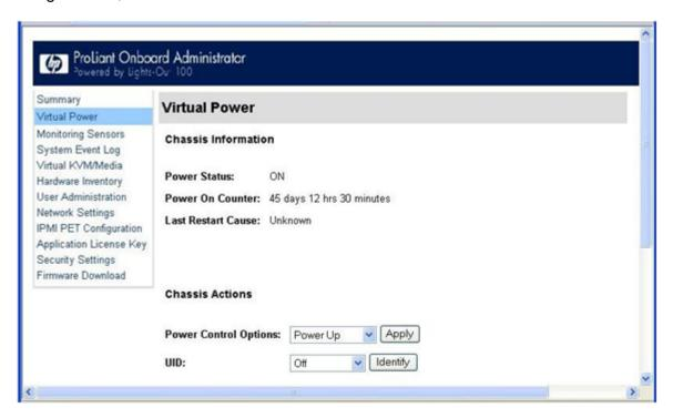
To modify Chassis Actions, select a Power Control Option in the Chassis Actions section, and then click **Apply.**
