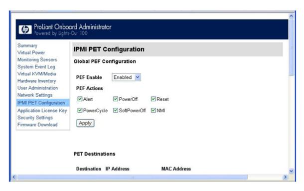
The Global PEF Enable section enables you to set a global PEF action. To create a global PEF action, select **Enabled** in the PEF Enable box, select the PEF action, and then click **Apply.**
