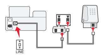
If the additional device (telephone or answering machine) has an RJ-11 connector, then you can remove the wrap plug and plug the device into the printer.
