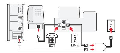
A Digital Subscriber Line splits your regular telephone line into two channels: voice and Internet. Telephone and fax signals travel through the voice channel, and Internet signals pass through the other channel. This way, you can use the same line for analog voice calls (including faxing) and digital Internet access.
