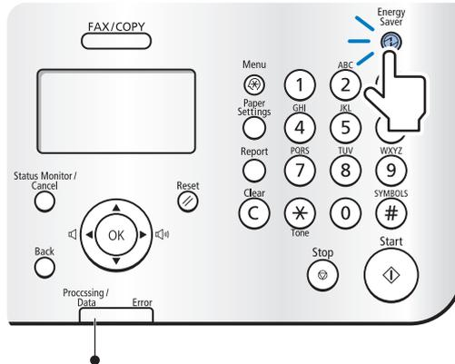
When the Processing/Data indicator is lit or blinking, the machine will not enter the Sleep mode, because an operation is in progress or an error has occurred.
