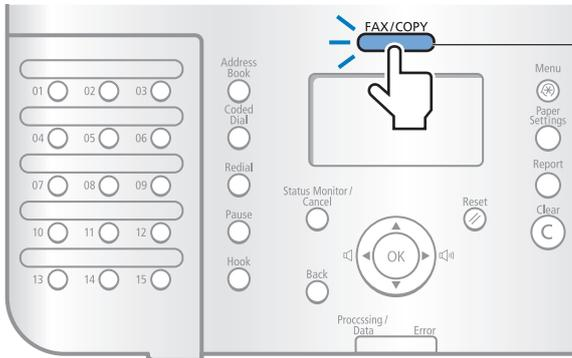
Press the key to switch between the Copy and Fax modes.
