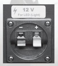
Your bandpass box also comes with another terminal that looks like the one pictured above. You need to hook this up to a 12 volt power source and a ground. The power (+) is on the right side and the ground (-) on the left side. You may want to wire this up to a switch so you can turn the LED light on and off. You can wire it up to the remote wire so the neon light turns on when you turn your stereo on.
