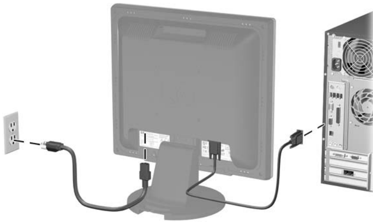
Figure 3-2 Connecting the Signal and Power Cables
