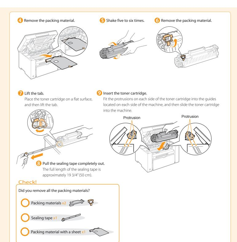
Preface Installing the Machine
