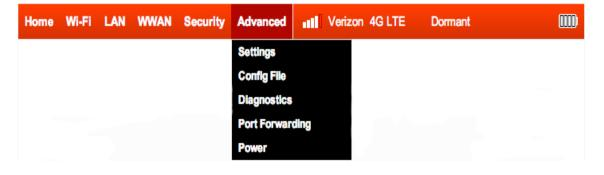
The Config File screen provides the ability to download (back up) a copy of the configuration settings from MiFi 4510L to a file on your computer, or restore (upload) a previously-saved configuration file from your computer to MiFi 4510L.
