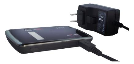
• Plug the other end of the wall charger into the appropriate electrical outlet. Charge for at least three hours.
