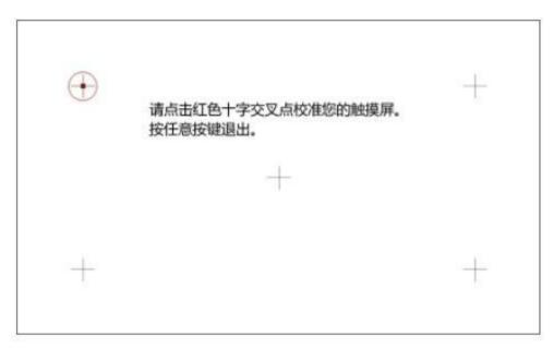
Use your finger or stylus to click on the intersection, click each one as per instruction, reboot the device, screen calibration setting complete.
