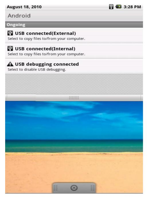
Click "USB connected (External)", select "YES" from pop-up Dialog Box, now you can manage all the files in Micro SD card. Click "USB connected (internal)", select "YES" from pop-up Dialog Box, now you can manage all the files in memory. After operation finished, turn off the Micro SD card/memory to remove safely.
