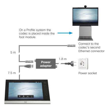
5. Verify that the touch screen is successfully connected to your codec by checking the codec address displayed in the top banner.
