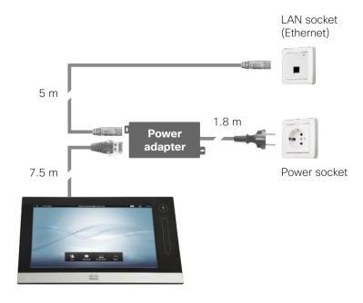
Note: The touch screen obtains its IP settings automatically from the network (DHCP). In most cases this is preferred and you can continue with the pairing.
