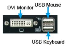
Plug a monitor into the Console's DVI connector; plug a USB keyboard and a USB mouse into the dedicated USB keyboard and mouse ports on the KVM switch. Ensure the keyboard/mouse are connected to the proper connectors.
